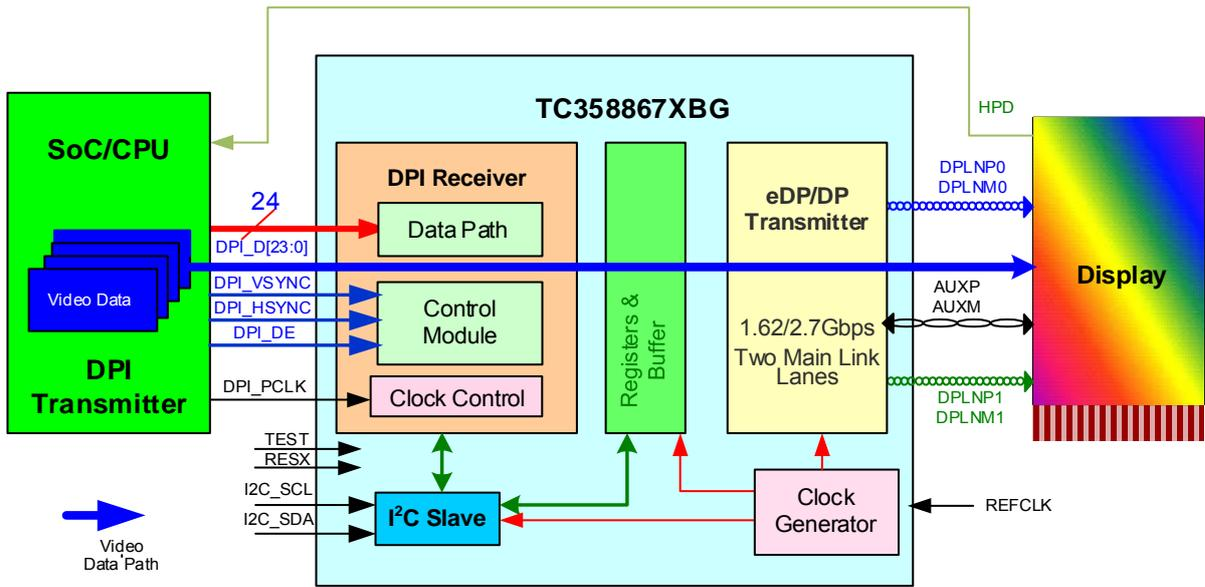
Figure 1.2 System Overview with TC358867XBG in MODE\_P21 Configuration
