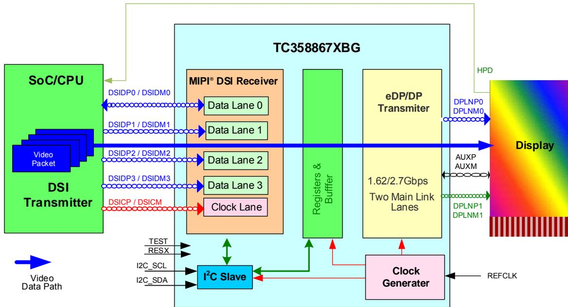
**Figure 1.1 System Overview with TC358867XBG in MODE\_S21 Configuration**
